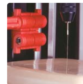
Simulated needle insertion smoothness test
